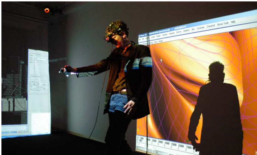
Figure 5. Media Lab for Augmented Architecture. The Lab contains an optical 3D Tracking System and an openly programmable set of sensors and advanced input and output devices (such as a head mounted display, high definition projectors and tablet screens).
