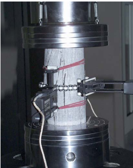
Figure 13. Failure by axial splitting along schistosity planes
