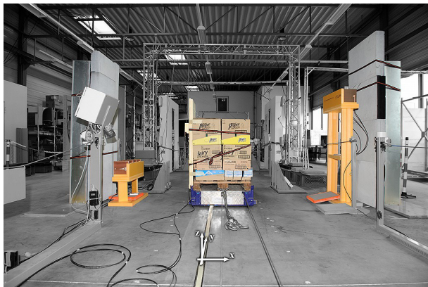
Fig. 8. Photograph of a gate setup with “ETSI” pallet (liquid cleaning agents in bottles) and absorber backplanes. The receiver antennas are mounted on the polyurethane foam slab left of the pallet. Note that the coordinate system is not at its origin.
