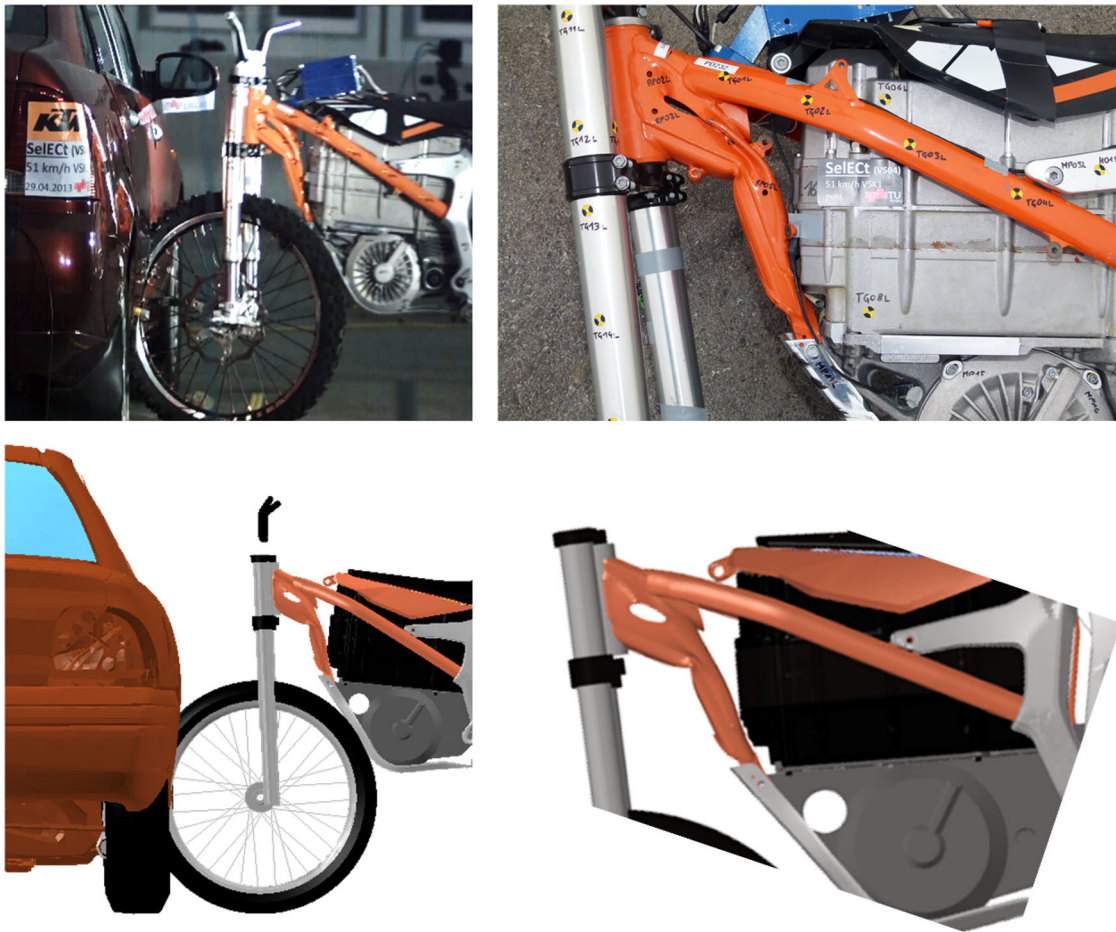
Figure 1. Most frequent motorcycle crash scenario (frontal collision of a motorcycle against a car): comparison of the test (top two pictures) and simulation (bottom two pictures) [37].
