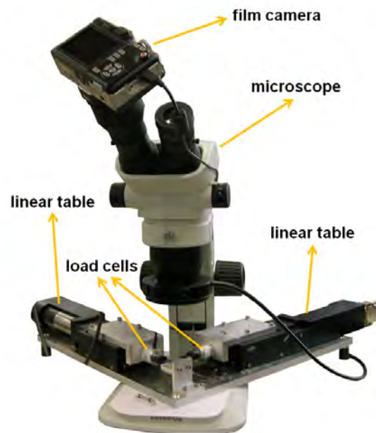
Figure 3.3 General view of the micro bond tester
