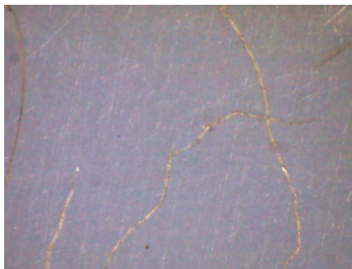
Figure 3.20 Fiber to fiber joint on teflon foil
