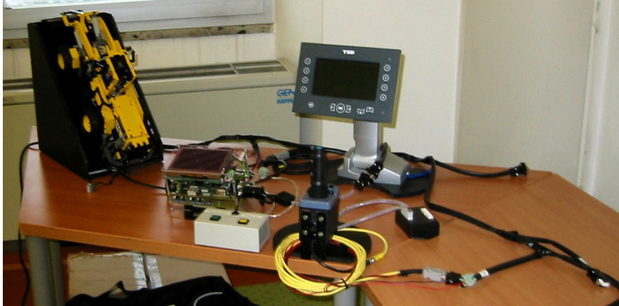
Figure 6.1: Demonstration setup of a wheel loader Lego model
