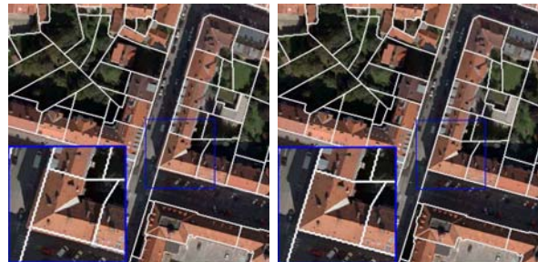
Figure 4: A cadastral vector data set is superimposed onto the true orthophoto for a segment of the Graz demo site. Note the small discrepancies between the data along property boundary lines manifesting themselves as visual feature in the imagery.
