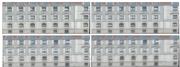
Figure 8: Of one single façade of the building in Figure 7 one will obtain multiple aerial image segments. These have been rectified into a façade coordinate system. From an aerial image block showing for each object point typically 10 images, not all will contain useful data for a specific vertical façade. Selected here are the 4 best, where "best" is defined as the largest area of a façade quadrilateral in the projection into an image.
