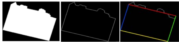
Figure 6: The classification layer “building” is based on color and texture. (a) shows the binary layer, (b) its contour in raster and finally in (c) the geometric figure of the footprint.
