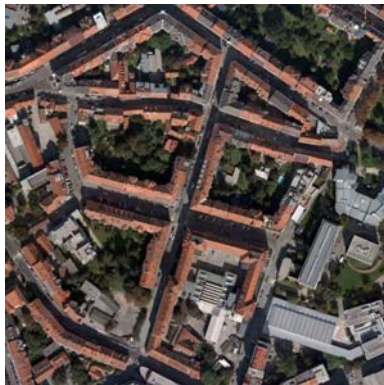
Figure 2: A 400 m x 400 m segment of an orthophoto of the urban core of the city of Graz (Austria). The pixel size is at 10 cm. The orthophoto is of the type “true”; therefore the facades are not visible.
