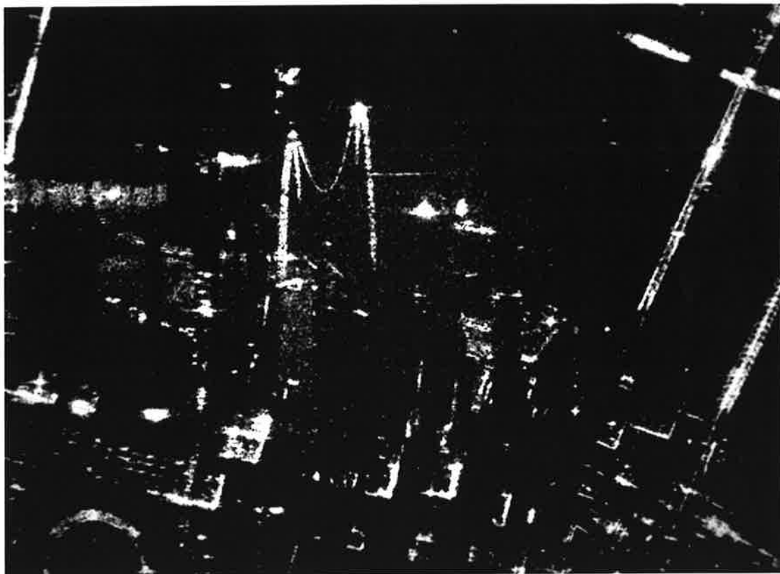
Figure 4-9. SAR image taken of the Gateway Arch with the GEMS-1000 radar system at X-band with ground resolution at 10 meters. Downtown St. Louis is at the bottom. The Mississippi and a few bridges are on the top of the image (courtesy G. LaPrade and formerly Goodyear Aerospace Corporation, now Loral Defense Systems).
