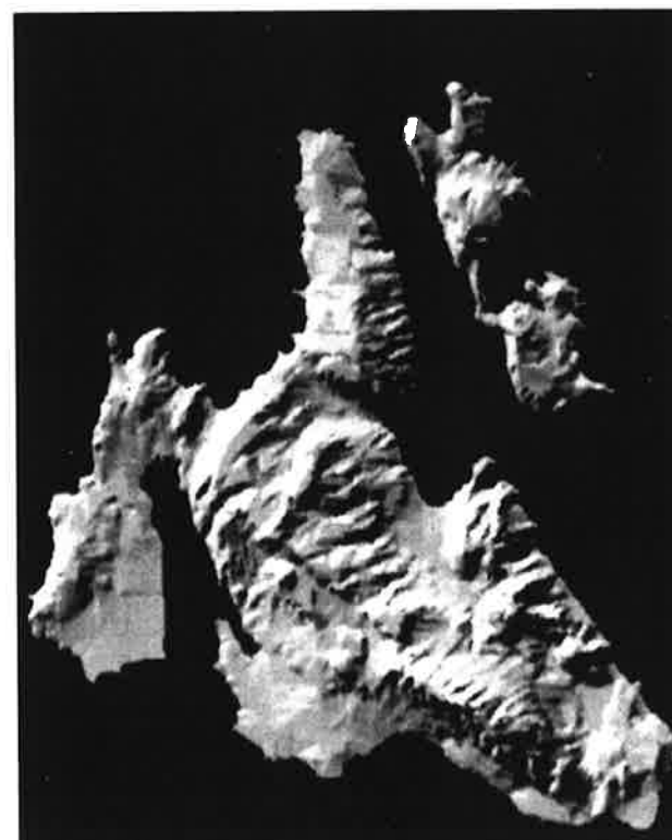
Figure 4-66. Comparing the squint-mode image with the undeformed (zero-Doppler) image. (a - top) Squint is 45^\circ but rectified (from Figure 4.65(b)); (b - bottom) Zero-squint image at 45^\circ rotated flight direction, to produce the same illumination as (a), but at a different geometry due to different azimuth. This image pair offers identical radiometry, but different geometry for stereo (courtesy G. Domik).
