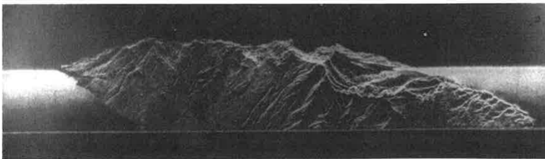
Figure 4-17. L-band (25 cm wavelength) SAR image of an island in the Atlantic, acquired by a NASA-JPL system. Slant range presentation covering about 10 km from the radar's nadir and sideways. Ground resolution about 10 m; flying height about 10 km (courtesy NASA-JPL).
