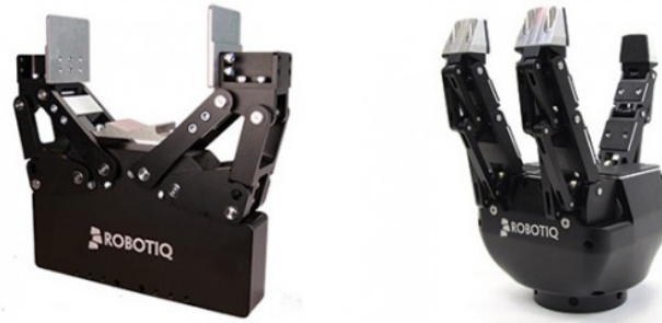
Fig. 11. 2-Finger and 3-Finger Adaptive Robot Gripper from Robotiq (Photo credit: Robotiq - Adaptive Robot Gripper)
