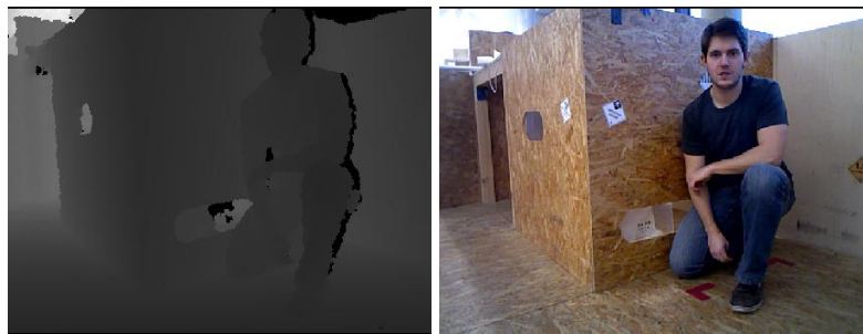
Fig. 17. Example for a depth image (left) and an regular image (right) of the same scene. (Photo credit: IST - TU Graz)
