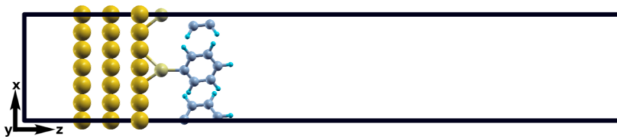
(e) A 8.86 \times 5.11 \times 50 Au|S|1P|H unit cell with three layers of gold was used in the convergence tests.
