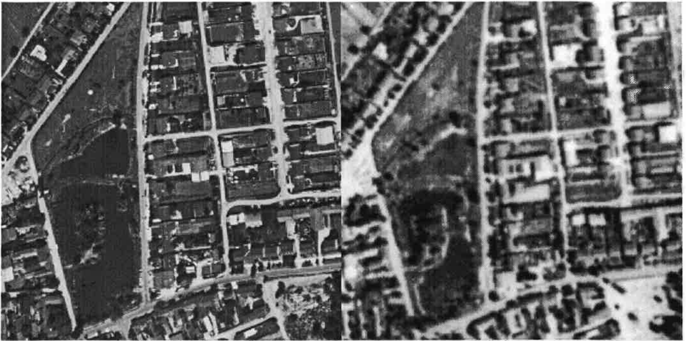
Figure 1: Comparison of sections of an aerial photograph 1:30,000 (2nd generation-product scanned) and right the same section from a Russian KFA-3000-image 1:80,000 (from 3rd generation-product). Area covered is 850 m by 850 m (1m pixelsize) in Illmitz/Burgenland. (Sindhuber and Herbig, 1994)
