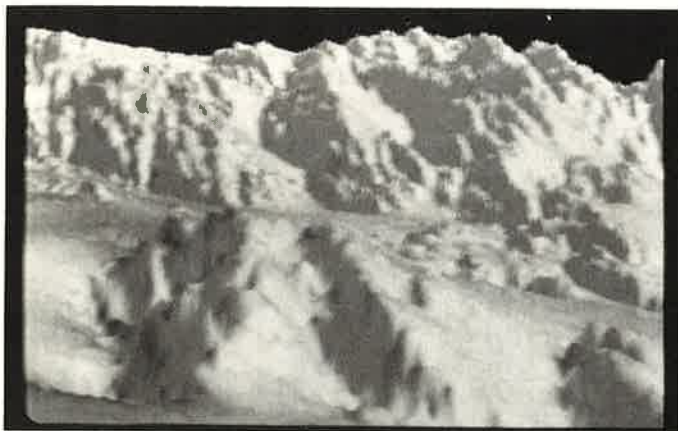
FIG. 20. Perspective view of the digital elevation model of the area in Figure 19, produced by shape-from-shading. Draped over the DEM is the image mosaic.
