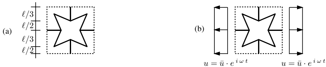
Fig. 1 Geometry and loadcase of the unit cell
