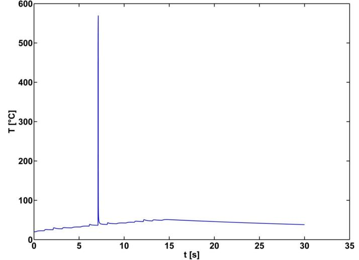
**Fig 6** Time temperature curve of the central weld spot (encircled spot Fig 4).
