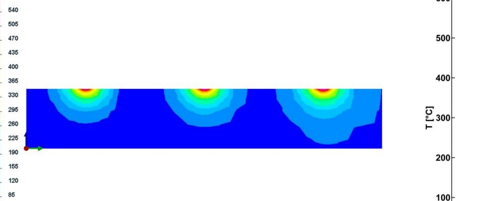
**Fig 5** Simulated temperature distribution of the central cross section (dashed line in Fig 4). The depicted temperature field represents the maximum temperature at each node during the computation. The welding order in time was from left to right.
