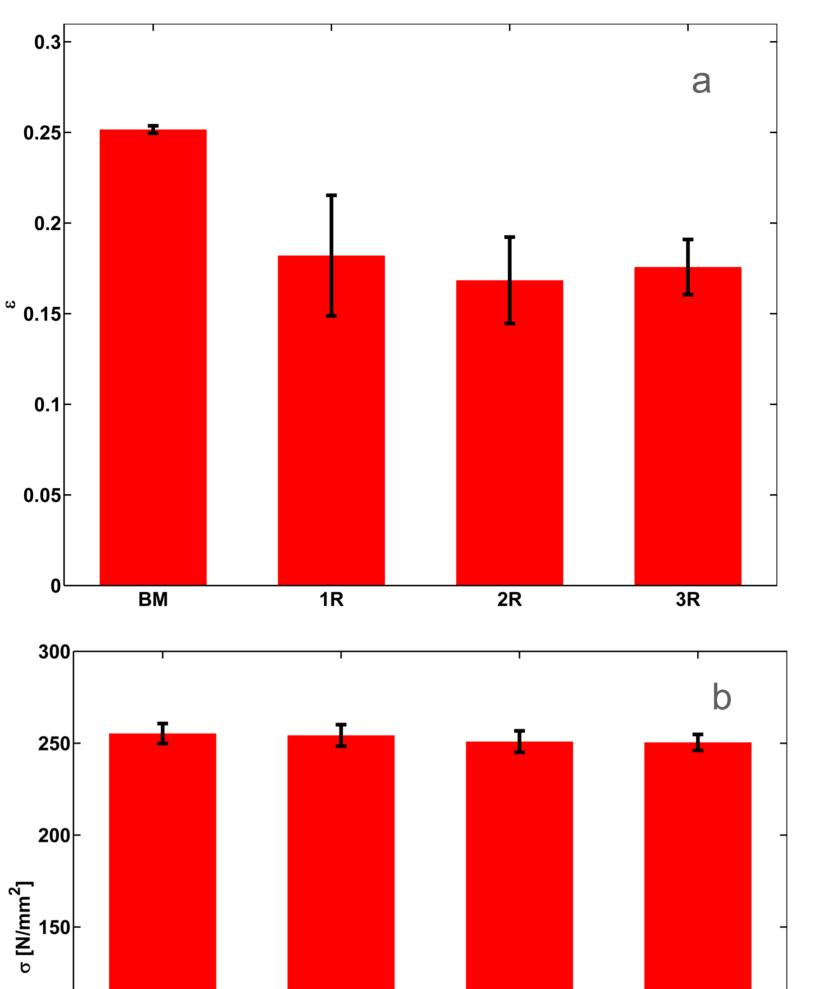
As Figure 2 shows, the ultimate strain decreases significantly after the pins were welded on to the plate. However, the ultimate stress shows no significant changes after welding.
