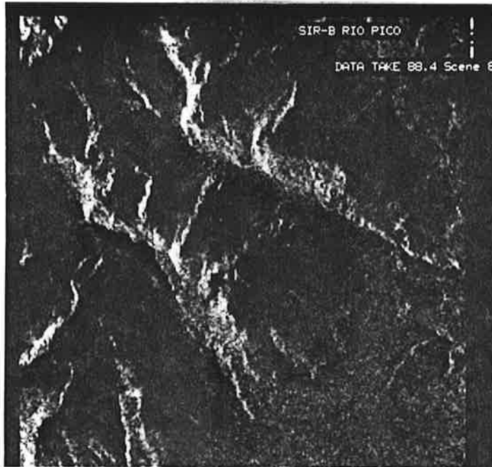
Figure 6: Raw SIR-B image segment (a), geometric rectification (b) and radiometric rectification (c), of an area in Gordón la Graza, Argentina. The black areas in the radiometrically rectified image are shadows. Coverage is 6.4 x 6.4 sqkms.
