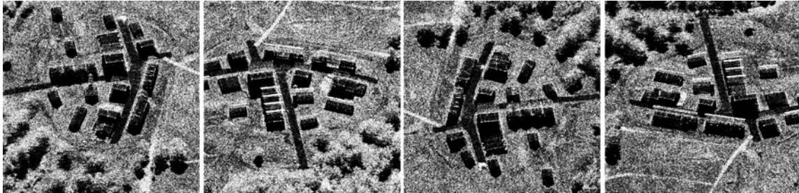
Figure 2: Synthetic Aperture Radar (SAR) test data set of a few rural buildings at a resolution of 30 cm per pixel and imaged from the 4 cardinal directions. The area covers approximately 220 x 220 m 2 . The images are presented with the flight line always from left to right on top (Courtesy Sandia).
