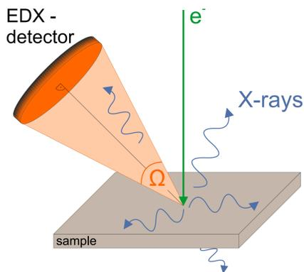
Characteristic X-rays are emitted in all directions, but they are only detected within the detector solid angle  $\Omega$ .
