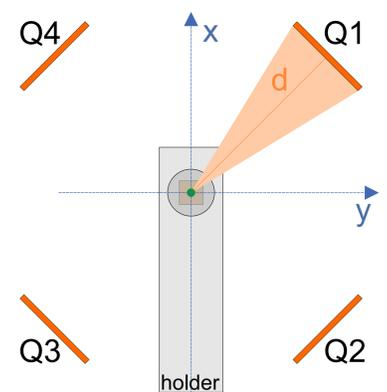
The Super-X detector: four detector-quadrants placed at a distance  $d$  to the sample.
