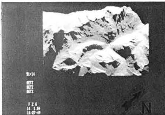
Fig. 7 : Simulated radar image : flight altitude 6 km, ground range presentation.
