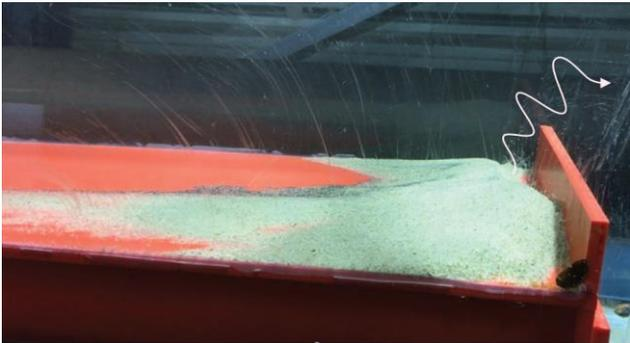
Fig. 7 Model test sand accumulation respectively to the prototype, visualizing of the vortex flow lifting sand particles ( [2], modified)
