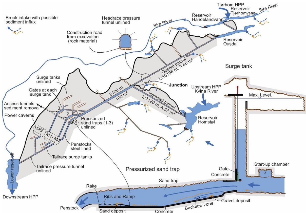
Fig. 1: Tonstad Hydropower scheme - characteristic Norwegian layout, surge tank with pressurized sand trap and proposed upgrade with ribs and ramp design.
