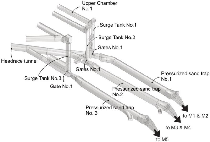
Fig. 2: Tonstad surge tank and pressurized sand trap system
