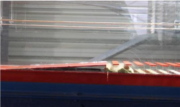
Fig. 8: Ramp and ribs solution for safely trapping of sediments as retrofitting proposal. Physical model test with 1:1 sediment and 1:1 velocity scaling ribs and ramp solution at weir ( [2])
