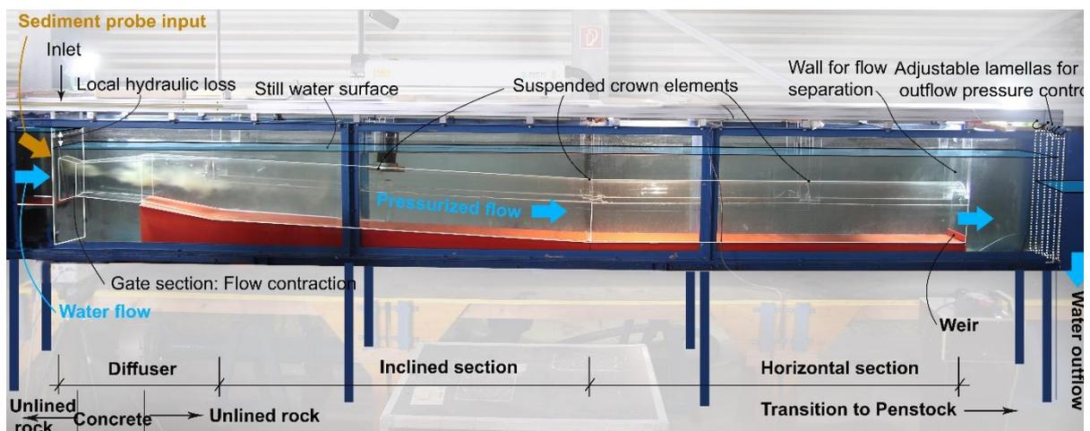
Fig. 5 The physical scale model test with 1:36.67 geometrical scale and 1:1 velocity and sediment scaling in the 30 cm wide flume of the hydraulic laboratory ( [2], modified)
