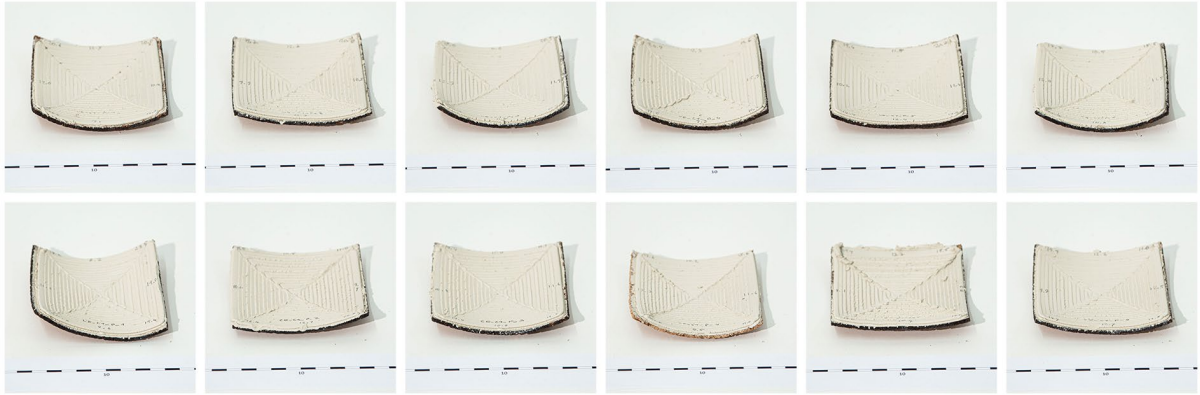
Figure 9: C1_P – paste-based extruded clay on cork 1
