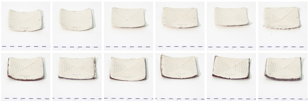
Figure 11: GF_P – paste-based extruded clay on Gautschfilz
