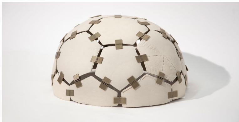
Figure 14: The final case study showing a dome structure made from multiple double curved elements
