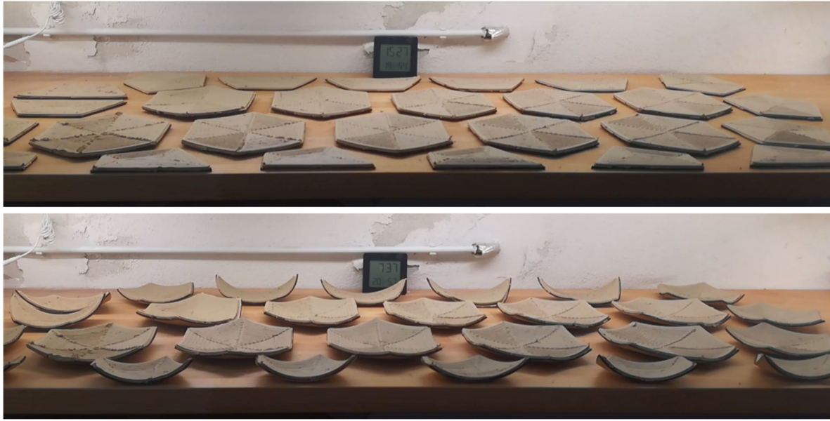
Figure 13: Elements for the case study: a) at the beginning of the drying process, b) at the point of reaching bone-dry state
