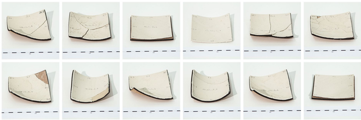
Figure 7: C2_M – manually applied clay on cork 2
