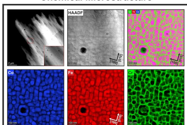
The chemical microstructure was determined using STEM imaging together with Co, Fe and Ni - EDXS elemental mapping.
