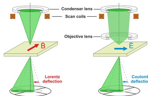
Magnetic and/or electric fields deflect the electron beam (Lorentz or Coulomb deflection). For magnetic measurements, the objective lens has to be switched off.
