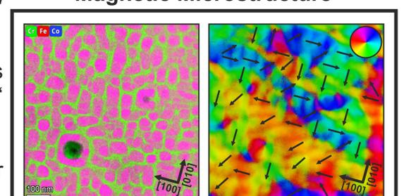
DPC measurements reveal the magnetic domain structure. Direct comparison with the overlay of the EDXS - elemental maps of the same region reveal the coupling of several FeCo-particles to form larger domains. The magnetization vectors within the domains tend to roughly point along the  $\langle 100 \rangle$  crystallographic directions.
