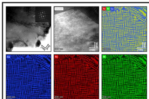
The chemical microstructure was determined using TEM BF and STEM HAADF images together with Cu, Fe and Ni EDXS elemental maps.
