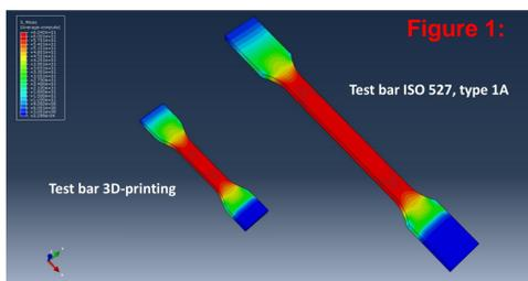
**Figure 1:** To improve the results of all mechanic analysis (static, dynamic, creep and fatigue), a separate test specimen was dimensioned especially for 3D printing parts. Small parts with the largest possible sample cross-section must provide comparable results to standard specimens, like test bar ISO 527, type 1A.
