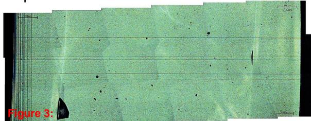
**Figure 3:** Stitched Light Microscopy image of a cross section of a FDM printed sample made of ABS.
