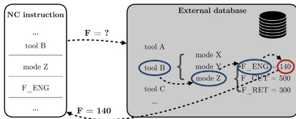
Fig. 5. Determination of feed rate through external database.
