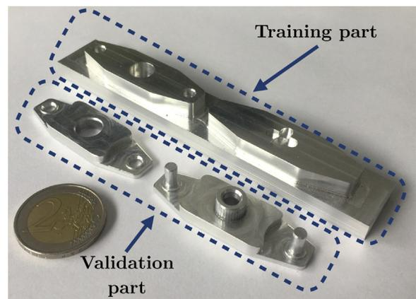
Fig. 3. Manufactured parts used for the study.
