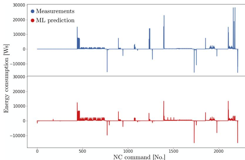
Fig. 8. Comparison of the prediction quality for the spindle aggregate for the whole machining cycle.
