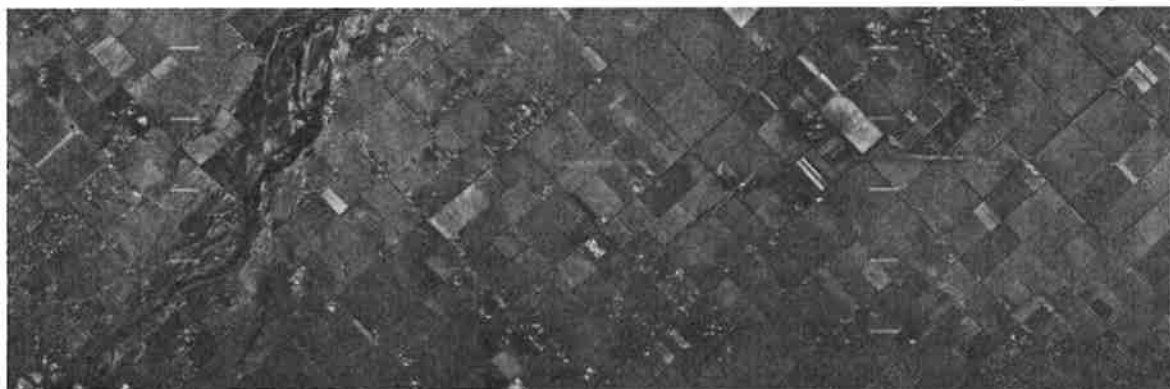
Figure 3 : Example of an aircraft radar image of an agricultural flat terrain. Flying height 12 km, radar wavelength 3 cm, resolution 3 m. Courtesy Geodyear-Aero-space.
