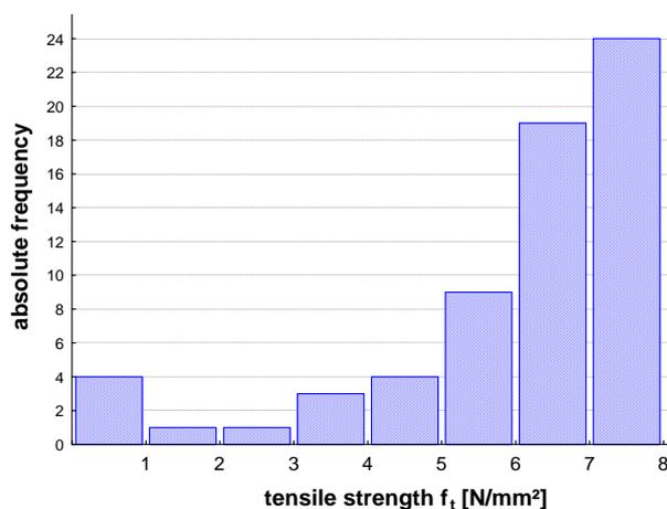
The frequency distribution of tensile strength of all broken specimens is shown in figure 3. Conspicuous is that near zero an accumulation is observed. This is because the specimens with nearly 'no strength' are related to faults of finger joints due to deficiencies in joint production. The rest of the lower tail of strength distribution shows the expected characteristic of rampant increase of failures with increased tensile strength.
