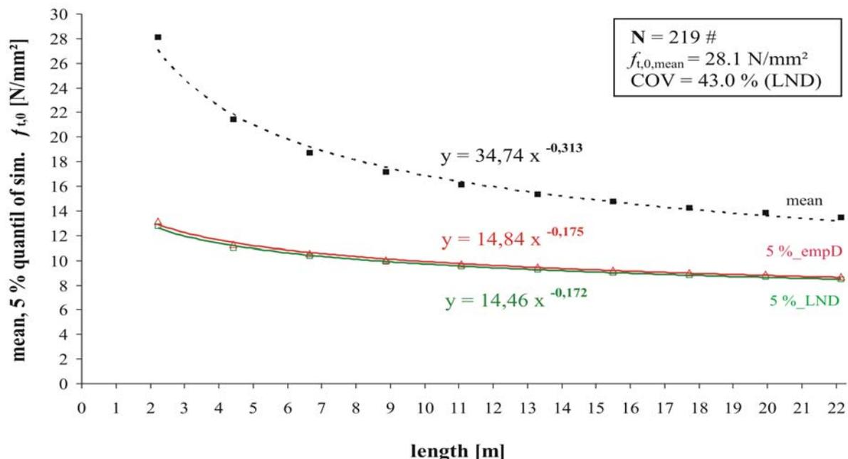
Fig. 8: Results of simulated length effect, based on test results of beams  $b/h = 60/200$  mm
