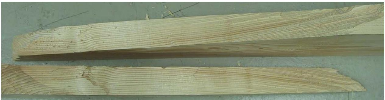
*Fig. 6: Tensile strength = 5,77 N/mm<sup>2</sup> due to reaction-wood and global grain deviation (Spec.Nr.1333)*
