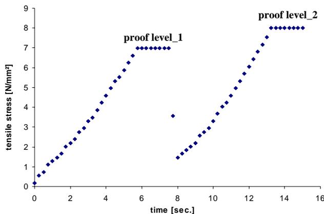
As illustrated in figure 2 first a proof level of 7 N/mm<sup>2</sup> and after a short relieve a proof level of 8 N/mm<sup>2</sup> was set. The speed of loading was, depending on the actual cross section, in the range of 10 to 60 kN/s and the proof levels were hold for at least 1.5 seconds. Within the total time of loading of about 15 seconds data (time, tensile force, extension of end grain) was recorded automatically at a rate of 4 Hz.
