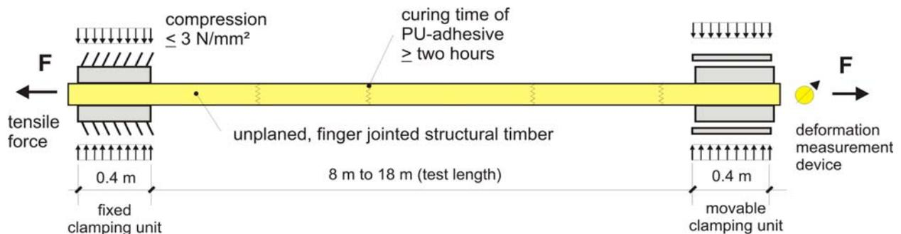
Fig. 1: System sketch of the tensile proof loading device for industrial application
