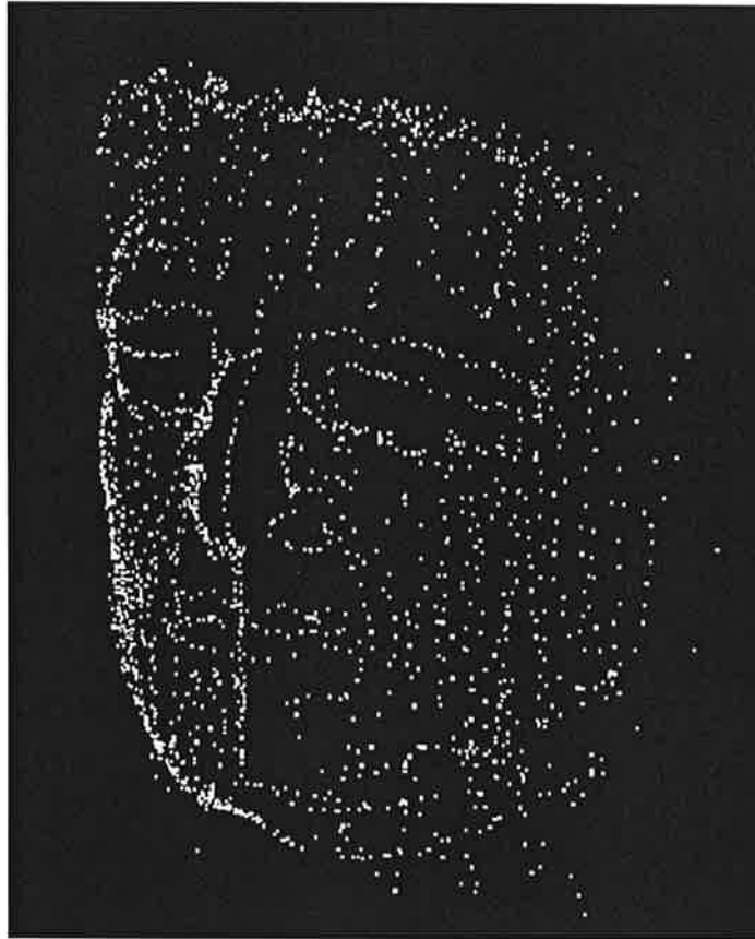
Figure 10 : Point cloud developed by the method describe in Figure 9 and obtained from a human face. Point accuracy is about \pm 0.5 mm. A set of 2000 points has been use to describe the face. Data collection is an interactive process taking about 600 seconds for this face.
