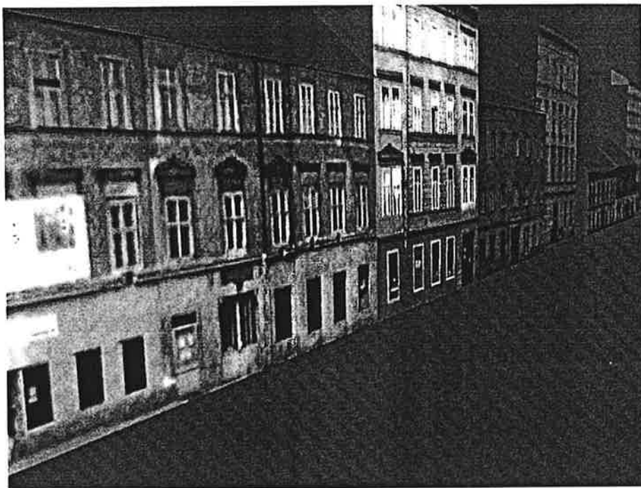
Figure 8: Perspective view of a segment of the 7th district in Vienna, obtained from aerial photography, Vienna's current GIS data, and augmented by phototextures extracted from aerial and terrestrial photographs. Total data set over one city block (4 street segments) contains 28 buildings along 560 meters of streets.
