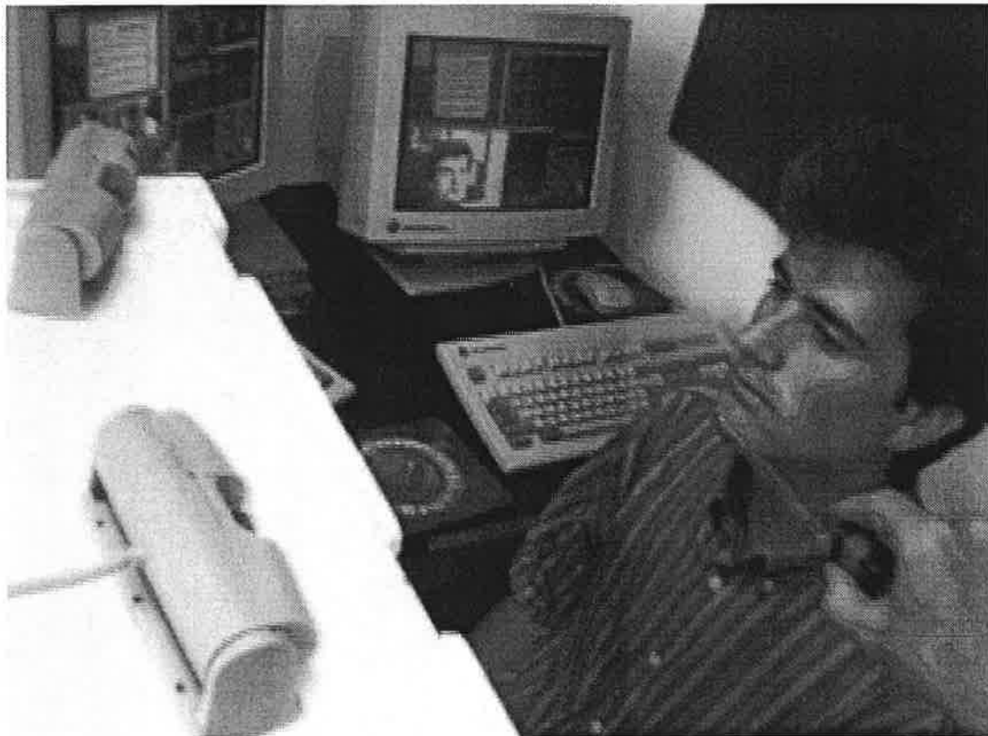
Figure 9 : System to model a face by means of tracking a colored pointer moving over the surface. The pointer is either an LED physically straddling the surface, or a projected red point obtained by a small projector pen used for slide presentations. Two cameras feed images into a Silicon Graphics Indy.
