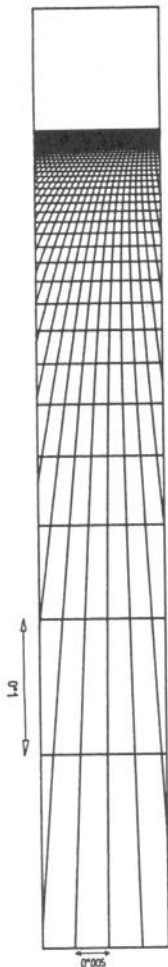
Figure 1a: Panoramic sector-scan geometry demonstrated with a scan from the horizon down to 60^\circ off-nadir. Focal length is 72", format is 5" x 36".
