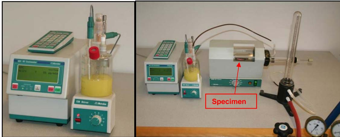
Figure 1 - Karl Fischer titration setup for moisture determination
