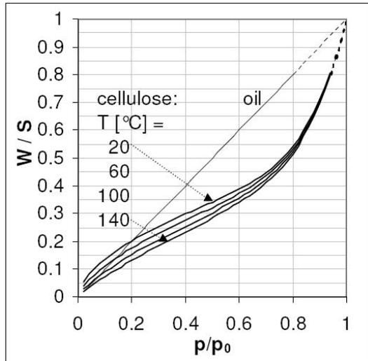
Figure 4 - Relative moisture in cellulose and oil [2]
