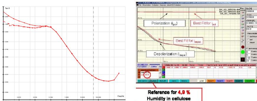
Figure 2 - Results of FDS and PDC Analysis
