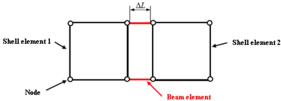
Figure 9: Scheme airbag cover modeling by using beam elements
