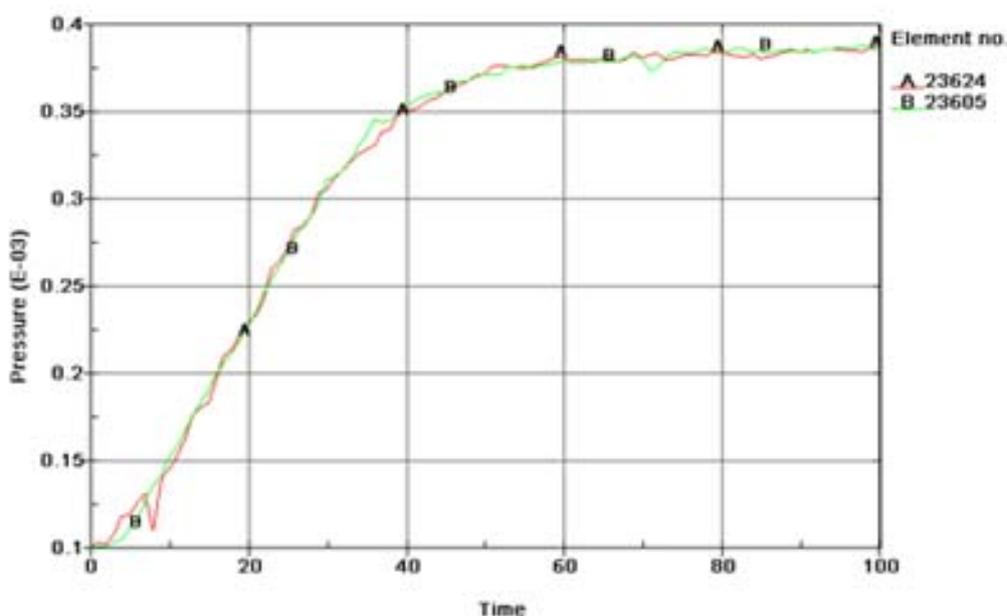
Figure 5: Simulated gas tank test pressure curve at ambient temperature and 100 ms delay
