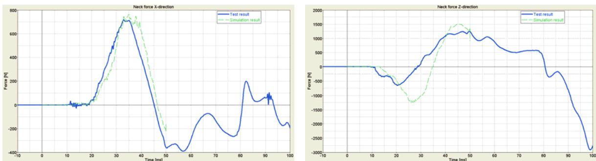
Figure 14: Neck force in X- and Z-direction
