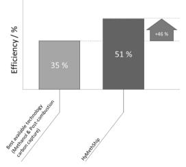
Fig. 2 Efficiency estimation for best available technology (methanol & post-combustion carbon capture) vs. HyMethShip (pre-combustion carbon capture)
