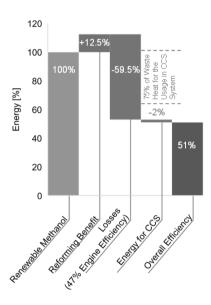
Fig. 4 Estimation of HyMethShip system efficiency
