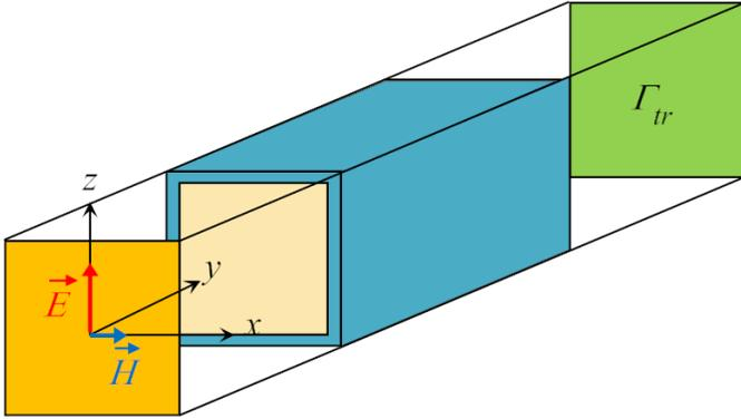
Fig. 2. Single wave guide, size =  $12 \times 12\text{ mm}$ , wall thickness  $1\text{ mm}$ .
