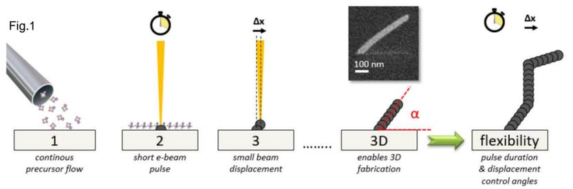
1. A precursor gas (chemical preliminary stage of the target material) is streamed into the vacuum chamber, where it physisorbs onto, diffuses along and desorbs again from the surface.
