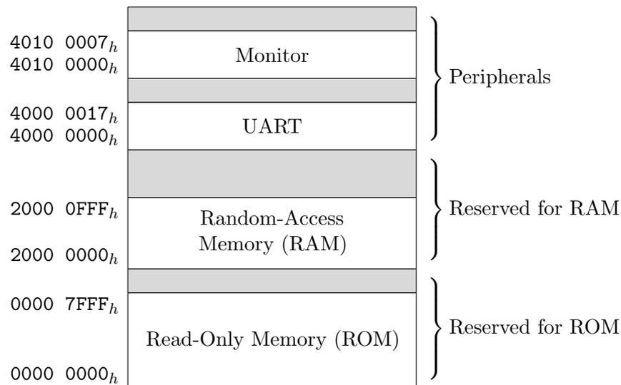
Figure 5.2: Address space layout with 32 KiB ROM, 4 KiB RAM, UART, and memory mapped monitor.
