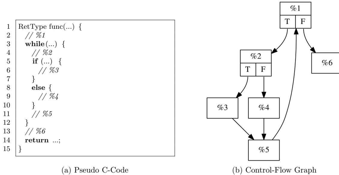
Figure 3.1: Control-Flow Graph example featuring a loop and branching
