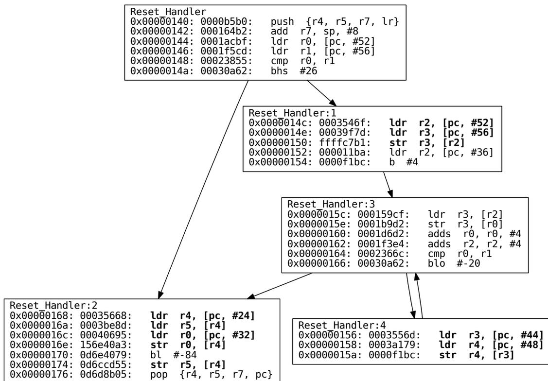
Figure 5.11: CFG from disassembling with signatures.
