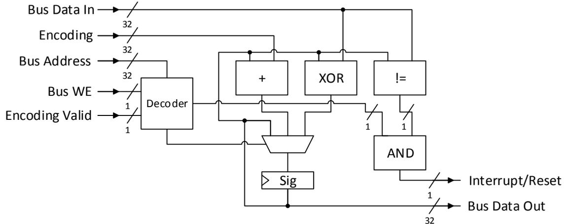
Figure 5.4: Structure of the monitor.
