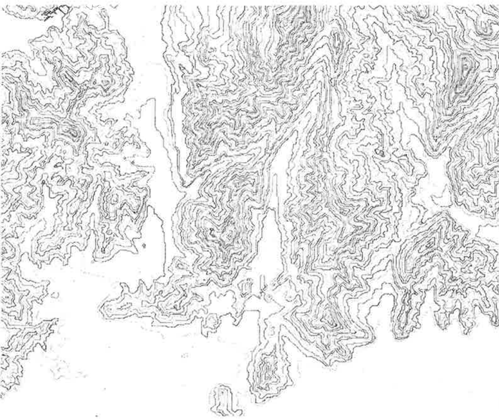
FIG. 18. Quality control of the height grid, using a rapid simple contour interpolation routine. The grid was generated using only contours.
