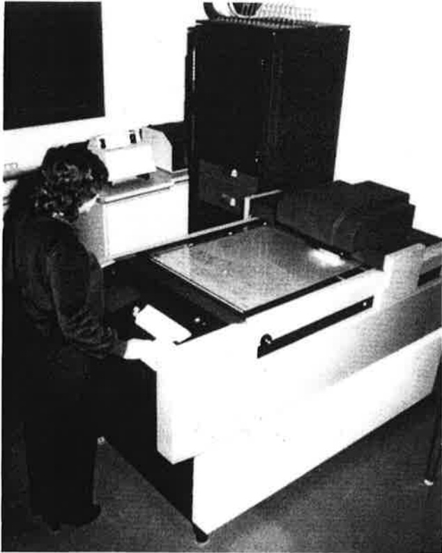
FIG. 7. KartoScan raster scanner in operation, recording output on magnetic tape.
