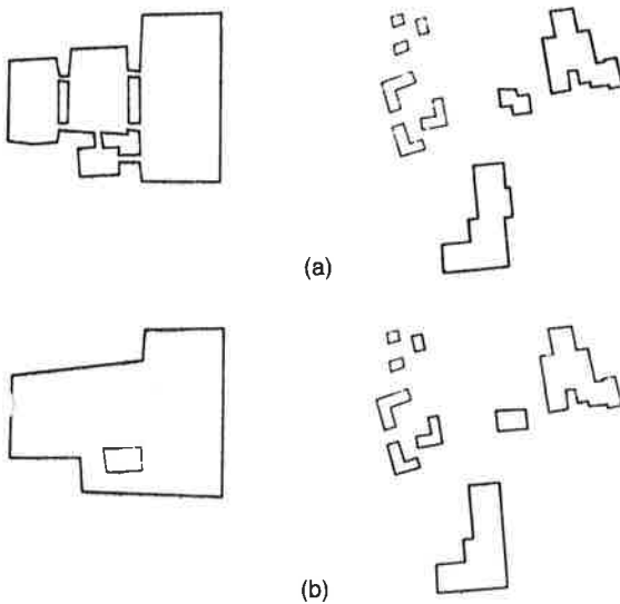
FIG. 9. Building outline simplification. (a) Raw 1:24,000-scale data (reduced to 1:32,000). (b) Generalized building outlines.
