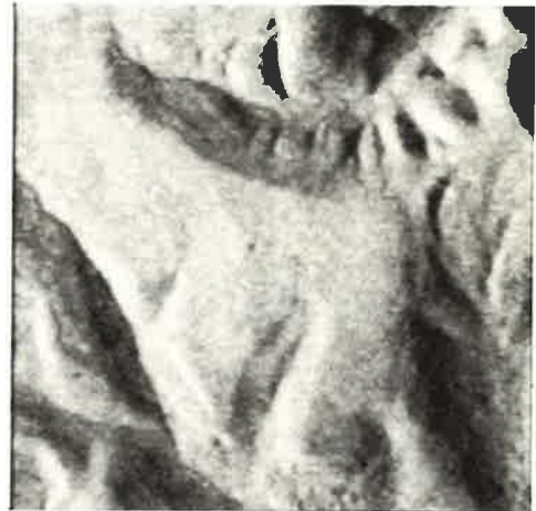
FIG. 5. Ortho-rectified input radar image. Same area as Figure 4, but imaged with a look angle off-nadir of 58°.
