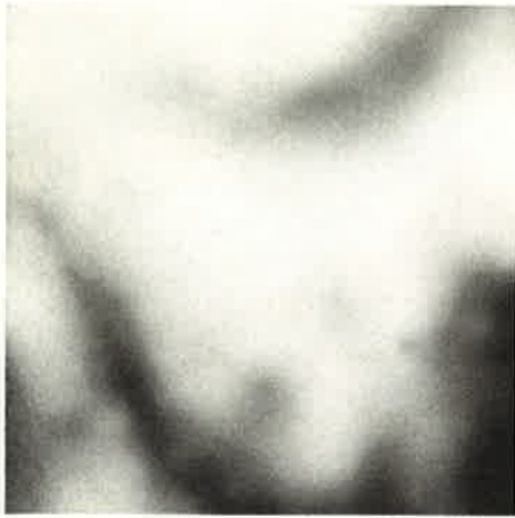
FIG. 11. Radar stereo height model with the heights linearly mapped into brightness values permits comparison with photogrammetric data set of Figure 10 (see also Figure 6).
