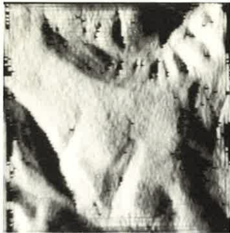
FIG. 7. Illuminated height model derived with radar shape-from-shading using as input the images in Figures 4, 5, and 6. Note the increase in detail when compared to the stereo-result (Figure 6) and the removal of stereo-induced artifacts. Striping along the area's edges is an artifact induced by "ringing" in the Fourier-Transforms.
