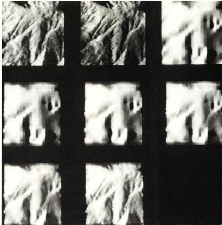
FIG. 15. Sequence of images to illustrate iterative nature of the shape-from-shading algorithm. (Top row, L-R: Input image 1, input image 2, illuminated radar stereo height model used as input. The remaining images are illuminated height models produced by shape-from-shading at 5, 10, 15, 20, and 25 iterations.)
