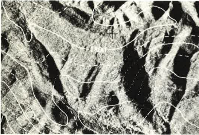
FIG. 1. Segment of a radar image map. Radar stereo derived contours superimposed over an image. Solid contour lines have a 100-m interval. Area covered is 5km by 4km. Note that contour lines do not model to smaller topographic relief elements, characterizing the coarseness of the stereo-based elevation. (Area: Brazeau Range, Alberta, Canada. Imagery: Intera Technologies Ltd., STAR-2, 6-m resolution, X-Band).
