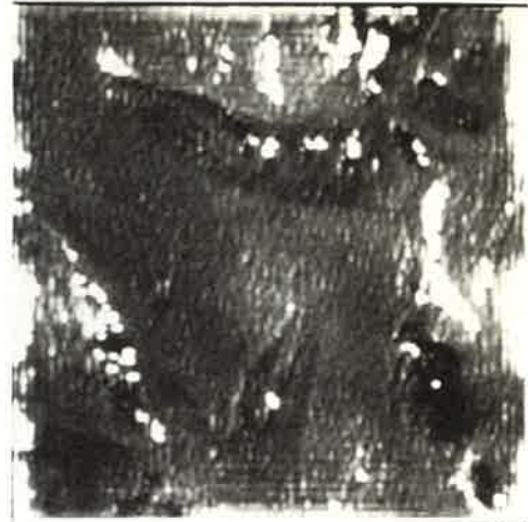
FIG. 18. This represents the same result as Figure 17, but employing the terrain slopes from radar shape-from-shading. Note that there is far less structure in this image than was found in Figure 17, leading one to conclude that the terrain slopes were more accurate than those used in Figure 17. The remaining areas of white exist where terrain slopes seem to be in error.
