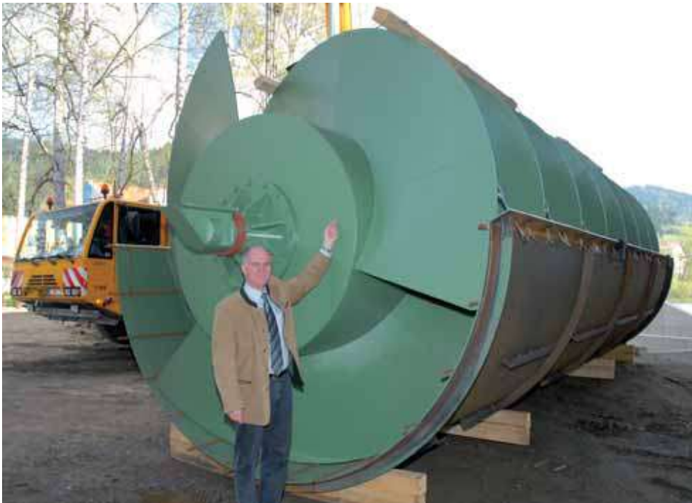
Figure 29: Hydrodynamic screw in Kindberg, with a diameter of 3.6 meters currently the world's largest hydrodynamic screw ( Kindberger Gemeindenachrichten, June 2008 )
