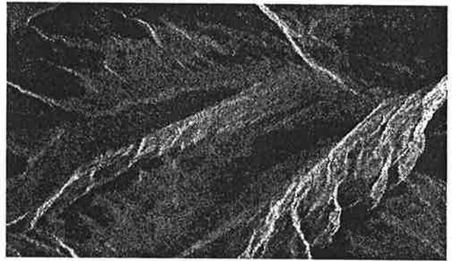
Figure 4: A simulated ERS-1 image of the scene shown in Figure 1. Multiple looks were incorporated by averaging three independently generated speckle files with Rayleigh random numbers.
