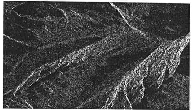
Figure 3: A simulated ERS-1 image of the scene shown in Figure 1. Speckle was simulated by generating one speckle file with Rayleigh random numbers of the same size as the simulated image and multiplying them pixel by pixel.
