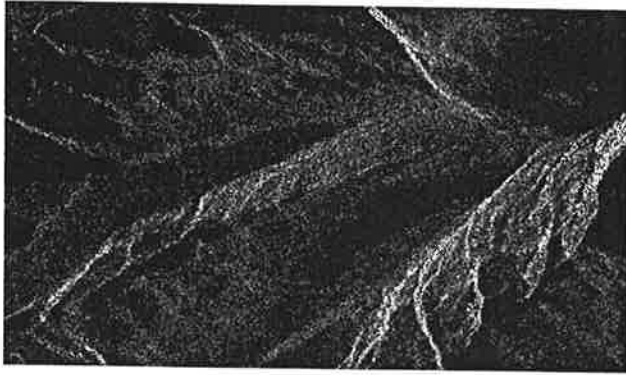
Figure 5: A simulated ERS-1 image of the scene shown in Figure 1. A chi-square distributed random number speckle file was multiplied pixel by pixel with the image from Figure 2. The number of independent looks is three.
