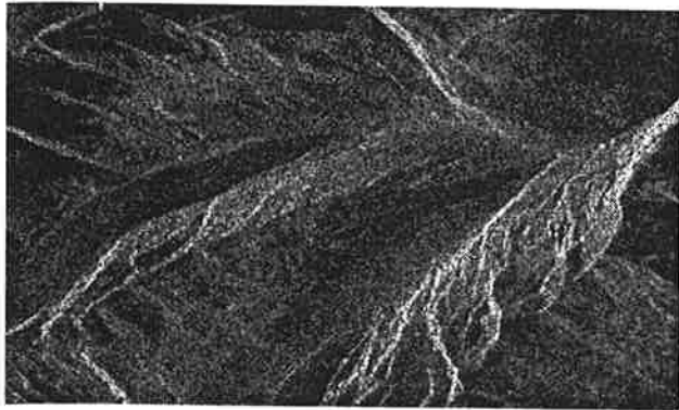
Figure 1: A detail of an ERS-1 scene of the Ötztal test site. The area covers approximately 9km x 5km. The scene was illuminated from the left, at a look angle of 23 deg. Copyright esa.
