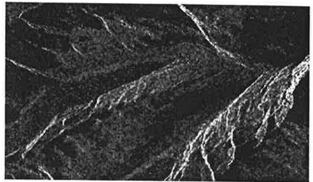
Figure 7: This image was obtained from Figure 2 by averaging three Rayleigh distributed speckle files, and applying a bilinear interpolation algorithm with a resampling coefficient of 0.5.
