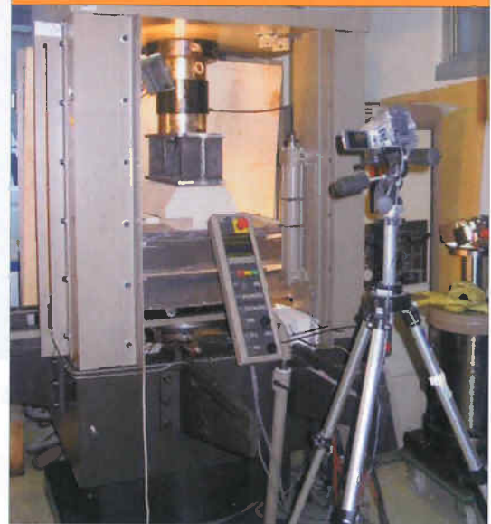
Figure 6. Test arrangement (compression frame) at rock mechanical laboratory of the Graz University of Technology.
