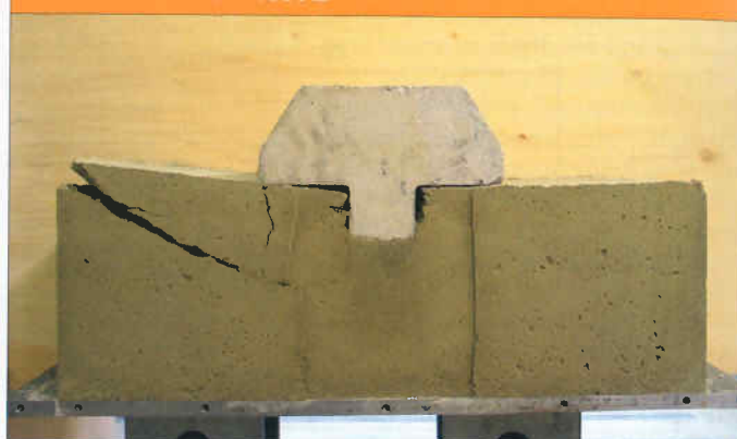
Figure 8. Penetrated ribs – test 2: UCS = 0.52 MPa.
