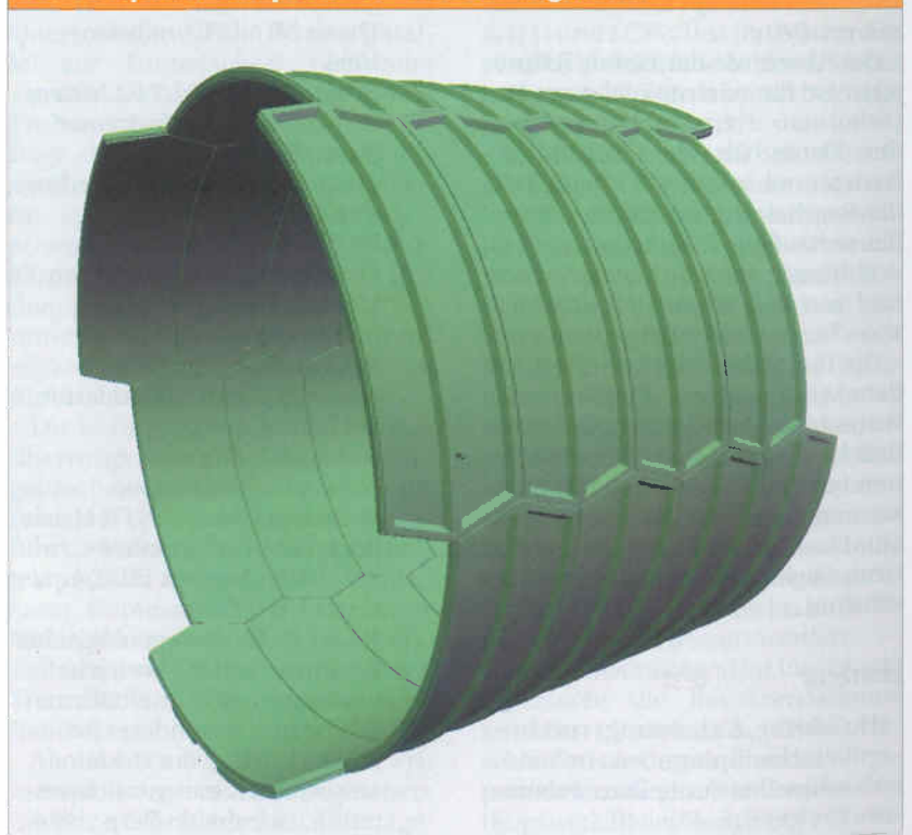
Figure 1. CO-CO System composed of »ribbed« segments [2].
