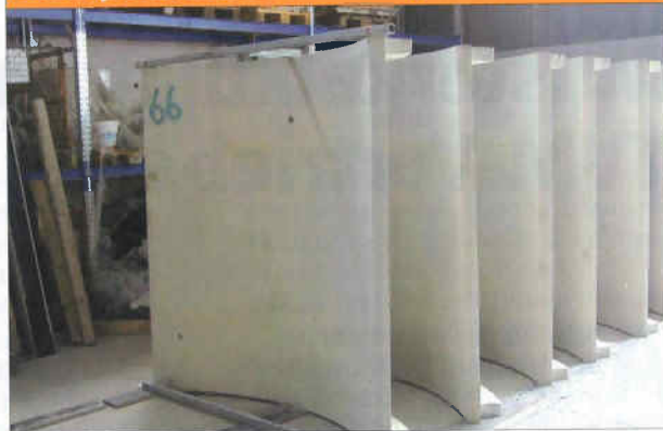
Figure 12. Serial production of ribbed segments.
