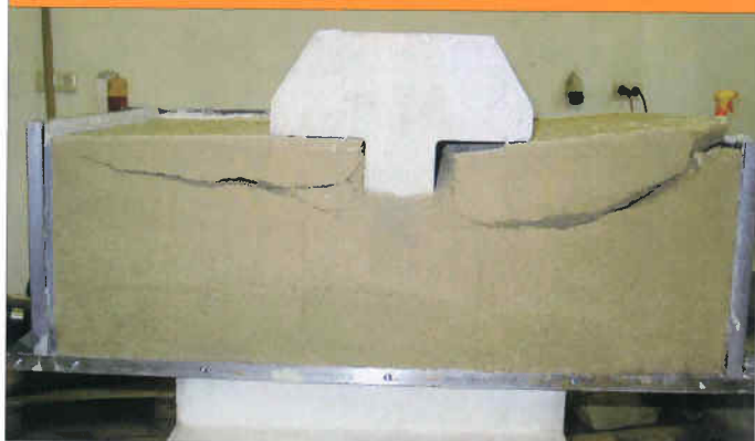
Figure 7. Penetrated ribs – test 1: UCS = 0.48 MPa.
