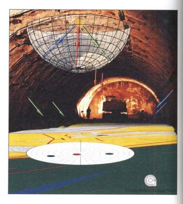
deformation patterns to the geological structure. The influence of rock mass structure on deformation behaviour is shown. Therefore it's a powerful tool to detect changes in rock mass quality well ahead of the face.
